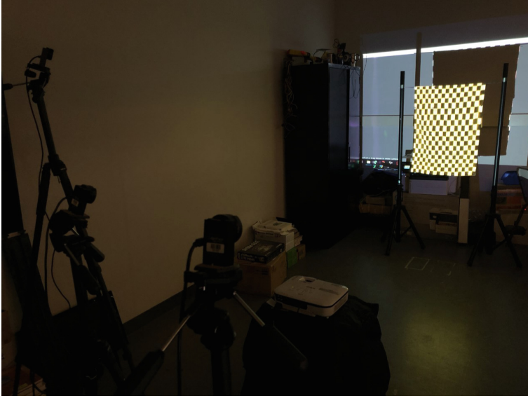
Fig. 5. Photo of experimental setup with three motion capture cameras, a projector and a towel being projected onto.
