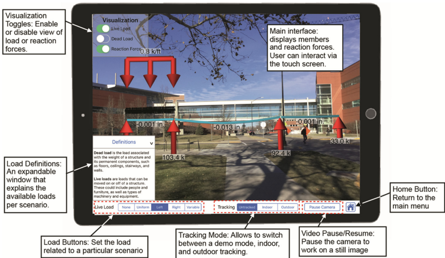
Fig. 2. The interface structure of iStructAR.
