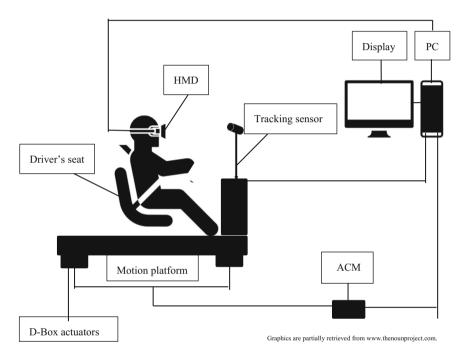
Fig. 1. The concept of VR driving simulation with HMD.
