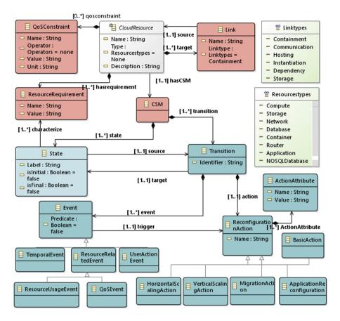
Fig. 2. UML class diagram for the Cloud Resource Description Model
