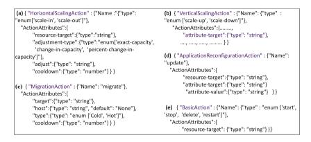
Fig. 4. A JSON schema describing the main attributes for each reconfiguration action
