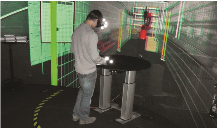
Fig. 4. HSI in SUTAVE-Lab on machinery with rotary table; floor marking tape to support safety zone detection.
