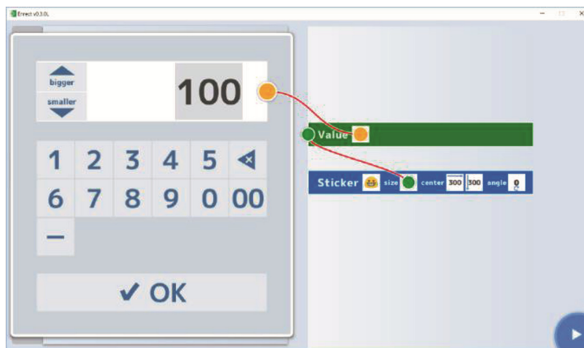
Fig. 9. In-app text input window connected to a parameter block with node-link interface.
