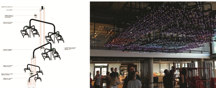
Fig. 7. Left: Exploded view of the clusters and cluster-to-supercluster assembly. Right: FLUID interacting with the audience within NEMO Science Museum
