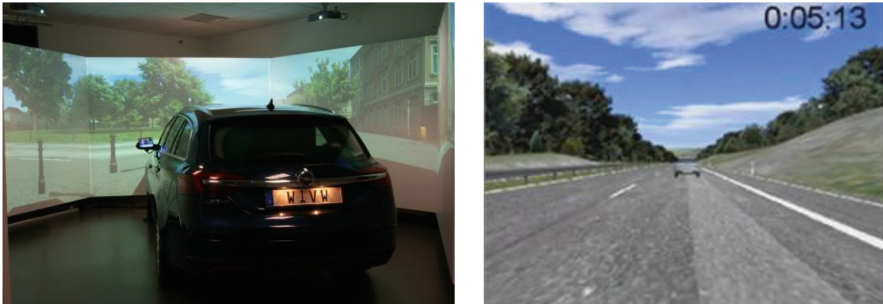
Fig. 1. Static driving simulator at the Wuerzburg Institute for traffic sciences and the car follow task (described in Sect. 3.2)
