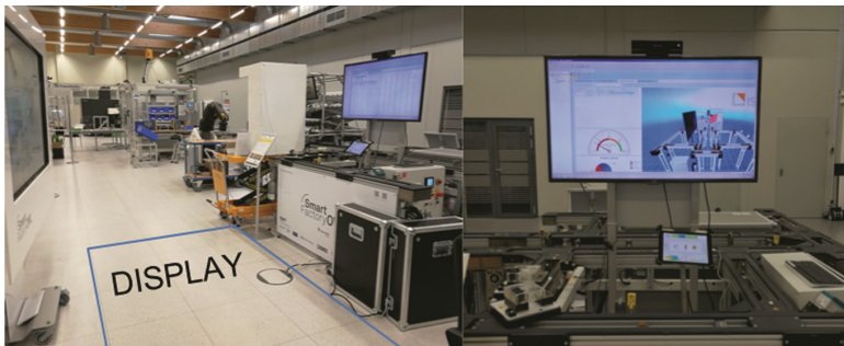
Fig. 4. Area of the third level localization in the SmartFactoryOWL (left). The localization is done by using a Kinect depth camera system on top of a display (right).
