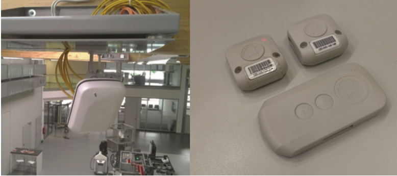
Fig. 3. A sensor of the UWB-system (left) and the associated tags (right).
