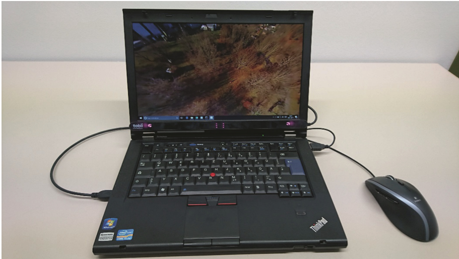
Fig. 2. Experimental system: image section displayed full-screen on a 14in laptop, equipped with a Tobii 4C eye-tracking device for gaze input, and a standard computer mouse providing the manual input alternative.
