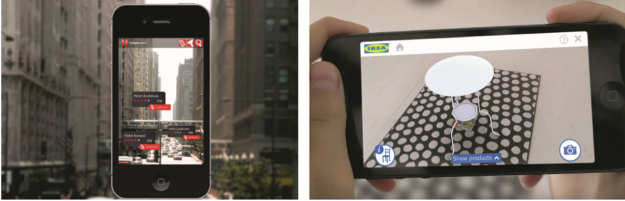
Fig. 2. Typical applications of mobile augmented reality: display of nearby points of interest (location-based AR) and visualisation of virtual furniture (image-based AR).
