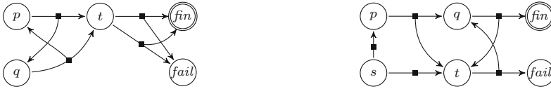
Fig. 3. Two target arenas with T = \{fin\} are shown. Round vertices are elements from V_P ; square vertices, from V_N . In the left target arena we have that p \sqsubseteq \{q\} and q \sqsubseteq \{p\} since any path from either vertex visits t before T —see Lemma 1. In the right target arena we have that t \sqsubseteq \{p\} —see Proposition 1.
