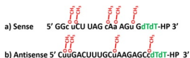
Fig. 10 Alnylam's RSV-modified siRNA. a siRNA sense strand 5'–3' 2'OME modified bases indicated in red; deoxynucleotide overhangs indicated in green; b siRNA antisense strand 5'–3' modified bases indicated in red
