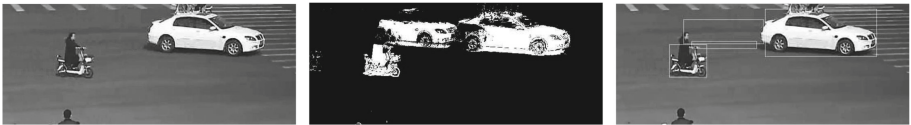
Fig. 2. Left to right: Illustration of the process of region proposal formation using GMM.
