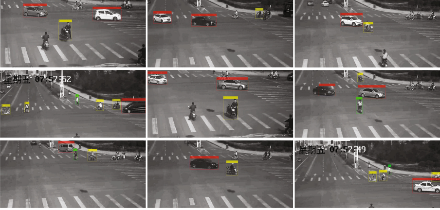
Fig. 5. Event verification at a road intersection. Three events are detected, recognized and labelled by a red rectangle (Event 1), a yellow rectangle (Event 2), and a green rectangle (Event 3). An object is detected when it moves; this generates an event to be classified; static objects are not labelled. (Color figure online)
