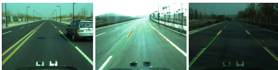
Fig. 8. Detection results for the proposed method. Left to right: vehicle, strong light, shadow
