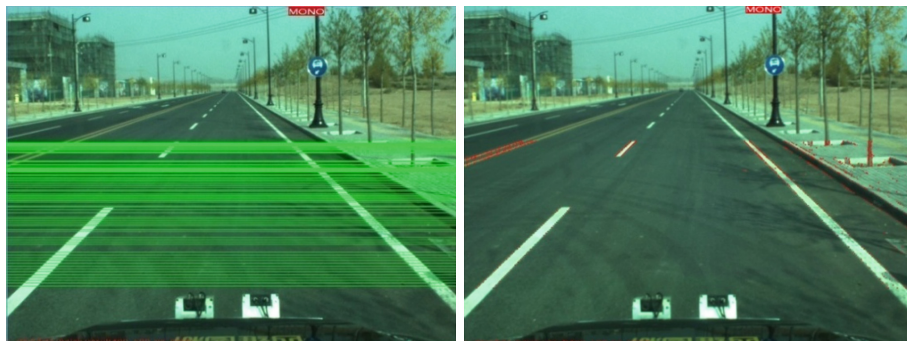
Fig. 2. Left: a set of scan lines. Right: examples of detected edge points; input image is as shown on the left
