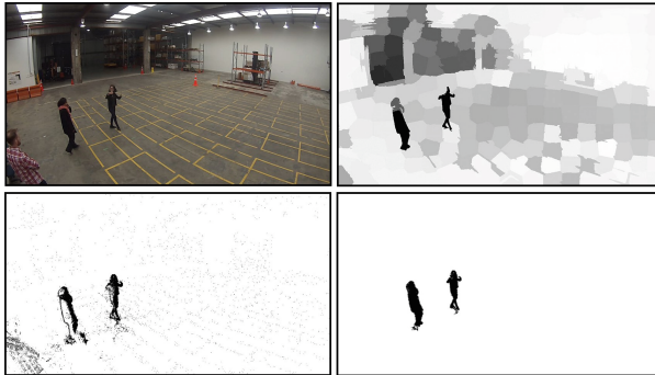
Fig. 9. Improved foreground based on pixel saliency. One of the pedestrians is missed, due to poor visibility both in MOG result and its saliency map
