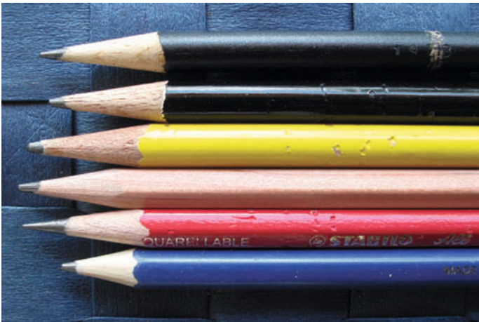
14.10 Wooden pencils with paint coating. The lead is embedded in a holder of Thuja , Juniperus and many other species.
