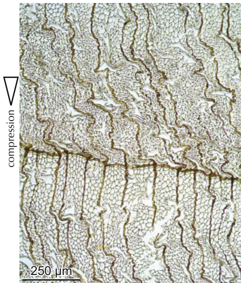
14.7 Compressed wooden structure of Populus sp. The intensity of the compression is reflected in the bending of the rays.
