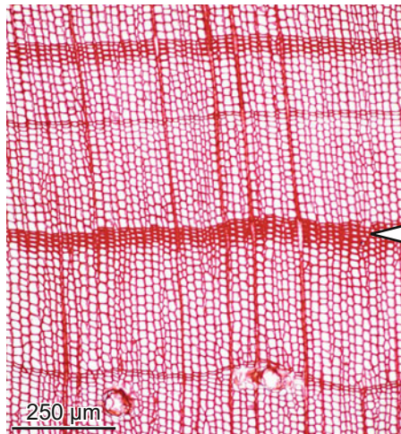
10.15 Individual ring with large latewood consisting of thick-walled tracheids in Pinus sylvestris .
