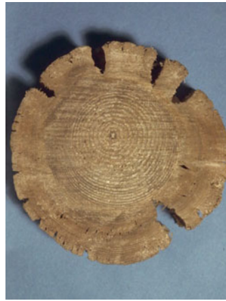
10.30 Large radial cracks in the anaerobically degraded peripheral zone of a Neolithic, waterlogged post of Abies alba .
