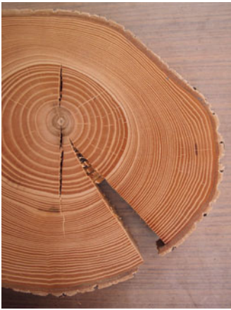
10.29 Radial cracks in a disc of Fraxinus excelsior are a result of intensive tangential shrinkage.
