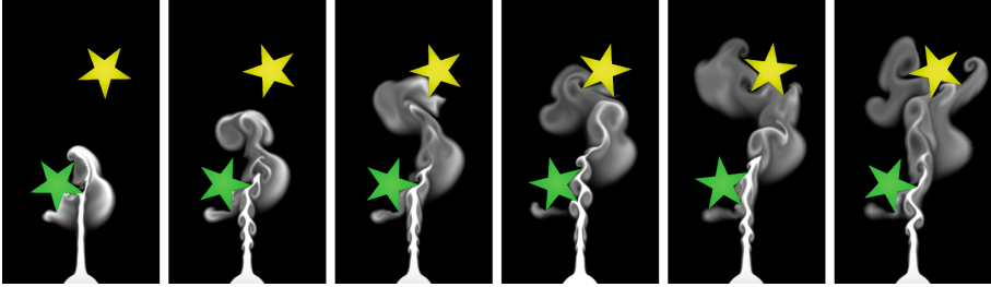
Fig. 3. These figures show the density of smoke at different time-steps. This simulation uses our method with the smoke injected from below. It processes at a resolution of 500 \times 900 grids scale and coupling with two rotating stars.
