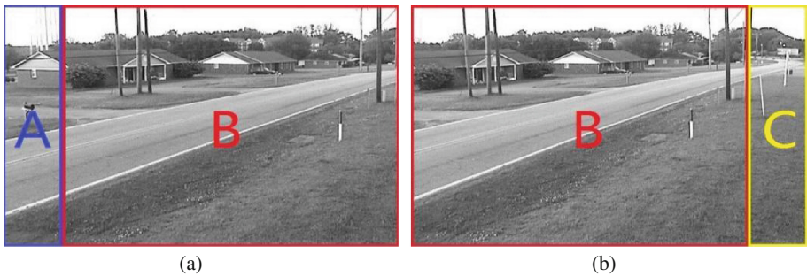
Fig. 2. Three parts of (a) a latter frame and (b) a former frame: region A (new background), region B (overlapping background), region C (disappeared background).
