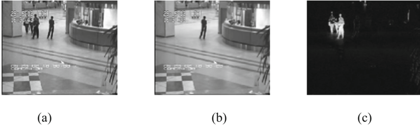
Fig. 1. Foreground extraction results based on PRMF-RPCA, (a) original image frame, (b) the low-rank component, (c) the sparse component
