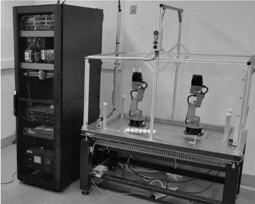
Figure 1. Robotic portion of the NIST ICS Cybersecurity Testbed.
