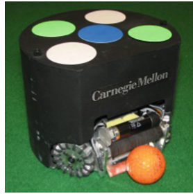
Fig. 1. CMDragon’s robot, with a ball touching its dribbler bar (horizontal black cylinder). The dribbling bar can be spun to put backspin on the ball for semi-control.
