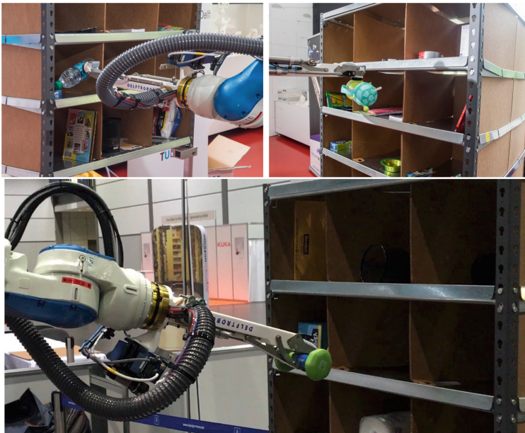
Fig. 5. The different gripper configurations for the grasping strategies. In the top images, the two configurations for suction rotating the cup. In the image below, the robot is picking the dumbbell using the pinch configuration.
