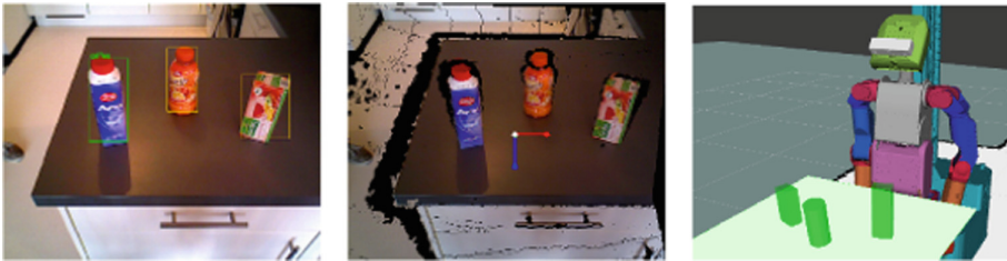
Fig. 5. The grasping pipeline. On the left output of the CLAFU component is displayed. The RVIZ environment including Floka, the detected planar surface as well as fitted superquadrics are visible in green. (Color figure online)
