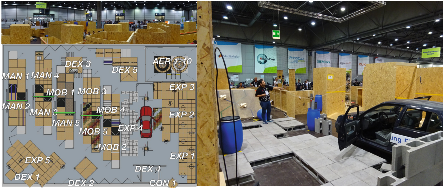
Fig. 1. Sample arena layout, showing the locations of all the test lanes set up for concurrent operation and a part of the real arena.
