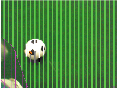
(a) Vertical scan lines and a detected ball candidate (the cross). Parts of the robot's body are ignored (bottom left).
