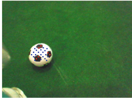
(d) The contour with the highest response (green) and the sample grid to check the ball pattern (pixels classified as black are shown in red, white pixels in blue).
