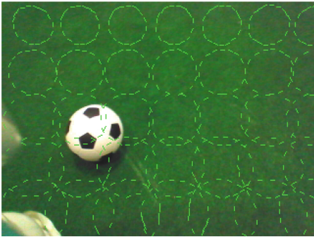
(c) Visualization of the search space for the ball contour. The actual search is only performed around the ball candidate, but in single pixel steps in both dimensions.
