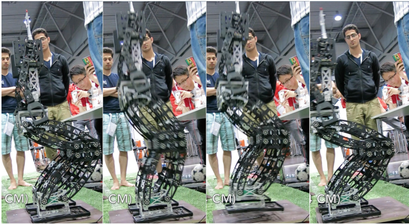
Fig. 6. Jump motion for 3.4 cm during the technical challenges, RoboCup 2016
