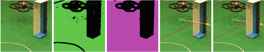
Fig. 4. The stages in processing each frame of a video to overlay the virtual drawings. From left to right: (1) the original frame, (2) the raw green mask, (3) the mask, after morphological operations, (4) the result of drawing without taking the mask into account, and (5) the drawing, masked appropriately. (Color figure online)
