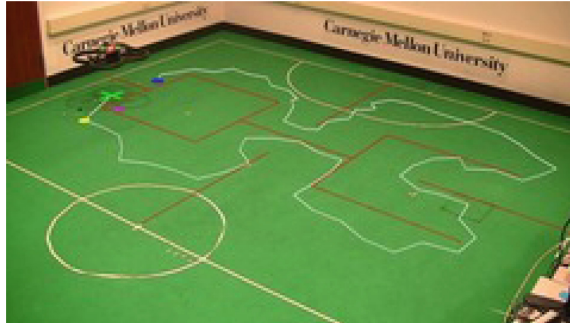
Fig. 5. The visualization generated from the RRT running with a domain consisting of entirely virtual obstacles.
