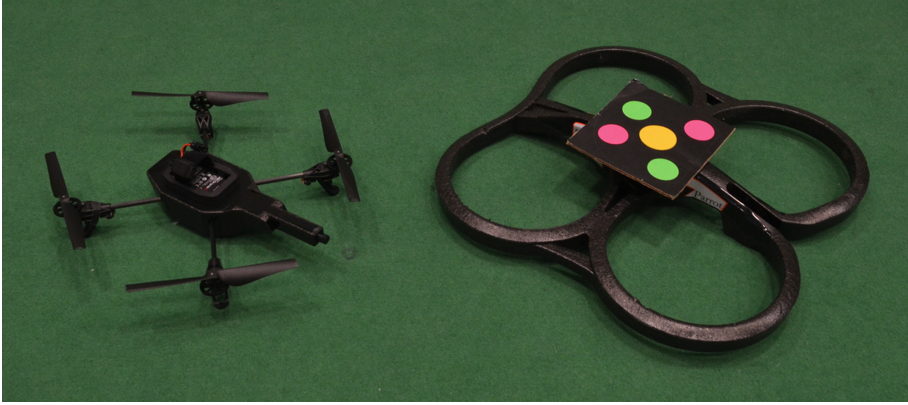
Fig. 1. The quadrotor we used to demonstrate our visualization, alongside its protective hull, which is used for safety when flying indoors. The colored pattern on top is not normally part of the hull; we used it for tracking (see Sect. 5). (Color figure online)
