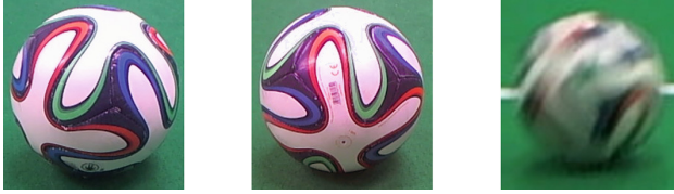
Fig. 1. One of the balls currently used in Robocup. The white color of the ball is almost identical compared to the color of the goal posts and the endlines. In the center image one can see the overemphasized red channel; this happens occasionally with our robot’s camera and the lighting in our laboratory. The left and center images show non-moving balls with a distance of 0.5 m to the robot. The right image shows a moving ball with a distance of 1.0 m to the robot. (Color figure online)
