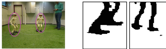
Fig. 3. Two non-green binary images for the detected robots in the left image. (Color figure online)
