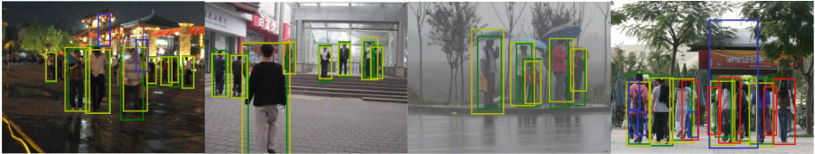
Fig. 2. Example DGHT + SCM + VGG16 detections on IAIR. (green): ground truth, (yellow): correct detection, (blue): FP, (red): FN; best viewed in color
