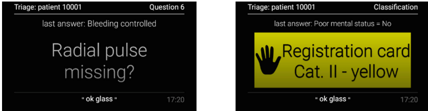
Fig. 4. Instructions and questions are shown to the user interacting via voice commands. (Color figure online)
