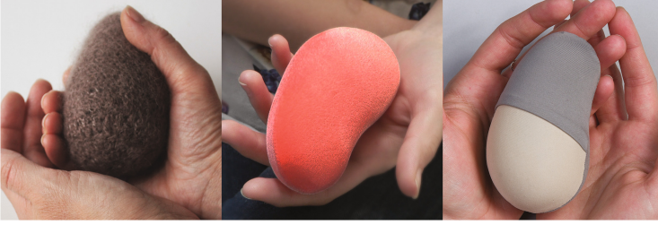
Fig. 1. Evolution of coating: knitted from wool (left), sewed from an elastic material (middle), easily exchangeable pattern sewed from an elastic material (right).
