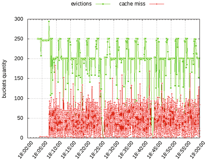
Fig. 6. uStorage iSCSI Target cache configured to 5 GB and set of files with 20 GB in total. The cache is four times fewer than the files we are storing. The algorithm is always making space on the cache with the eviction (bucket remove) operation and all the Cache Miss (restore) operations never overlaps the quantity of evictions .
