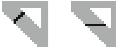
Fig. 1. Two homotopic openings (black) for the same object (gray) with the same size. This example shows why we cannot judge a homotopic opening by its size.
