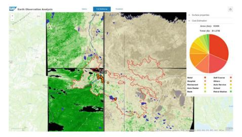
Fig. 2 Change detection based on NDVI
