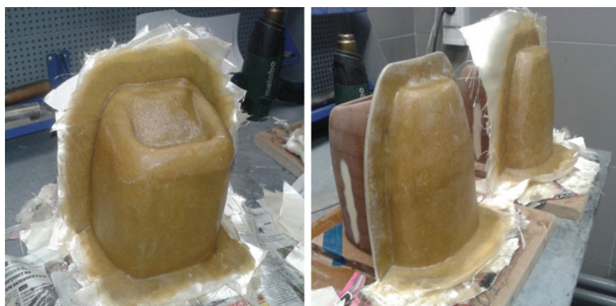
Fig. 3 Forming tool. a bottom matrix, b top matrix)
