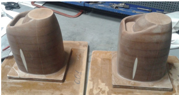
Fig. 2 Master model nacelle of hood
