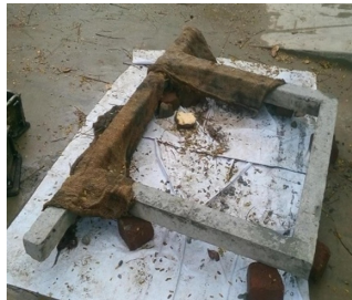
Fig. 10. Casted RC framed specimen
