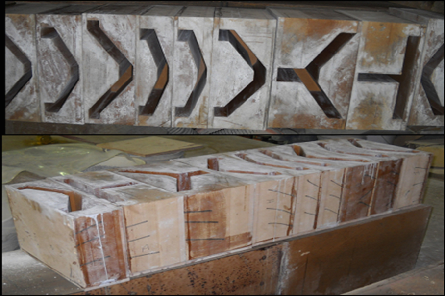
Fig. 6. Wood moulds used to cast the flat and shell footing models
