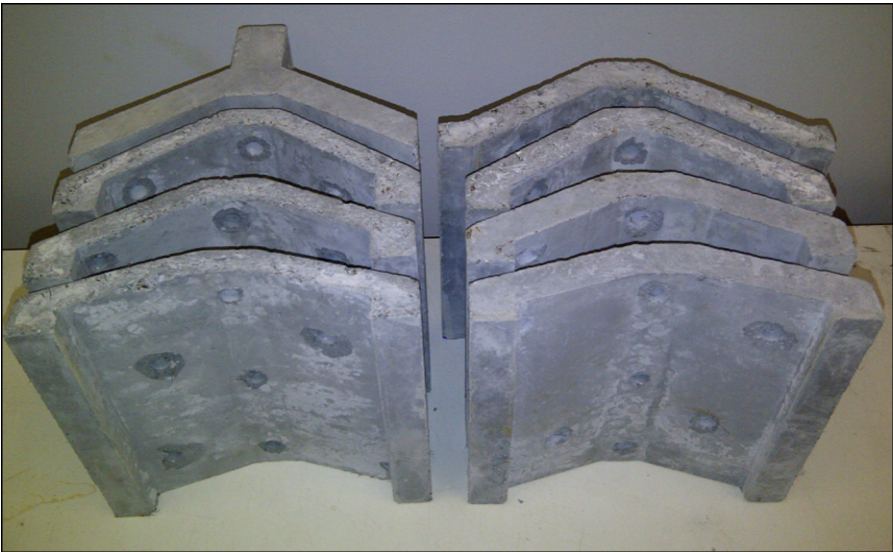
Fig. 7. Overall view of casted shell footing models made of mix concrete
