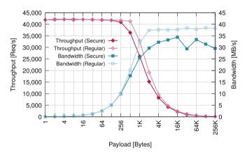
Fig. 6. Request throughput and traffic for various payload sizes.
