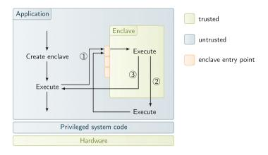
Fig. 2. Interaction between untrusted application and SGX enclave.
