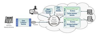
Fig. 4. Architecture of the dam monitoring application SGX-enabled
