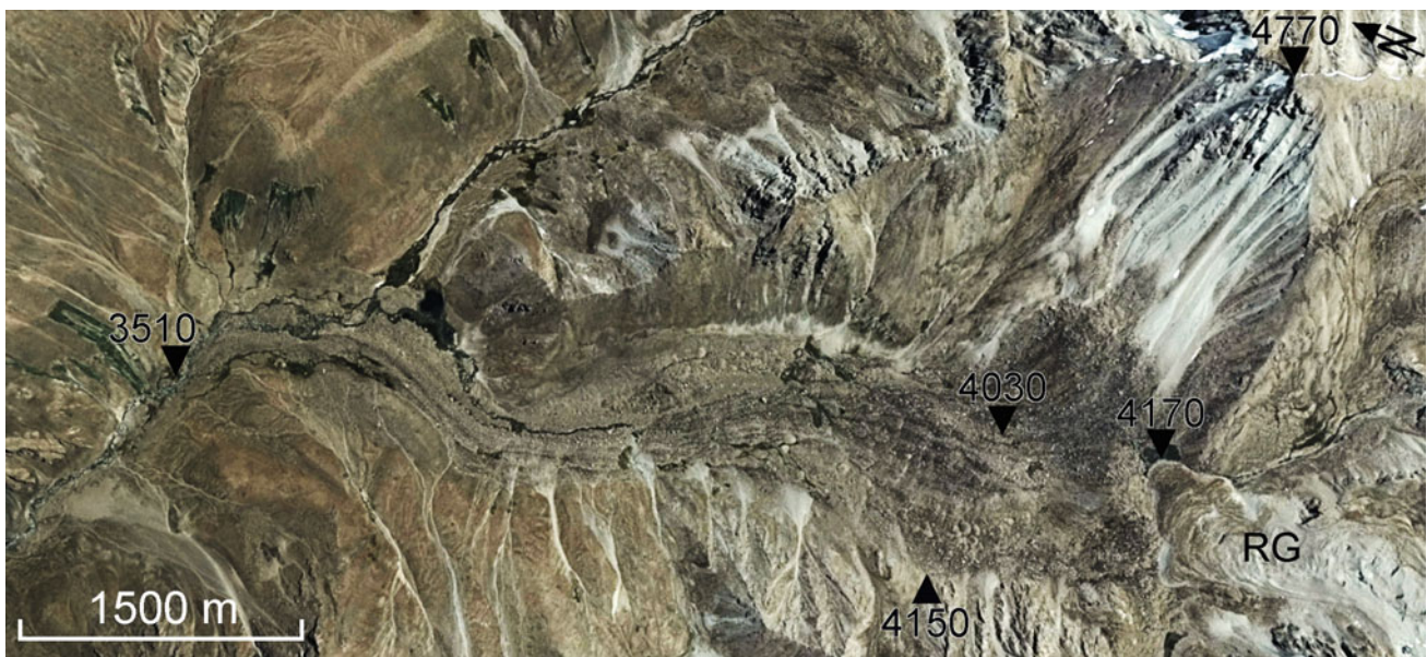
Fig. 6 The 5.5 km long Urmochdara rock avalanche in the Gunt River basin (South-western Pamir) with the striated microrelief of the deposits indicating flow-like debris motion. RG—rock glacier with a totally different morphology
