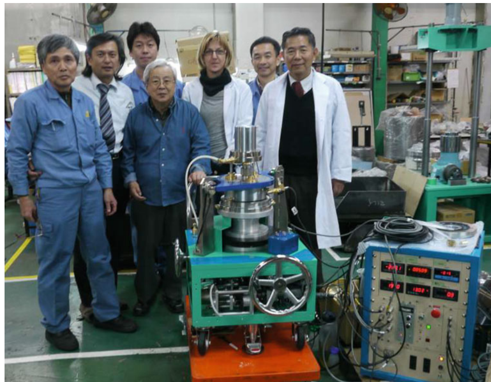
Fig. 7 Photo of developed transportable undrained dynamic-loading ring shear apparatus in the factory of the producing company. (At the center front is late Takeshi Nakasono, chief designer of the apparatus, at the center in the back is Maja Ostric, invited from Croatia, who obtained her Ph.D. based on the development of this apparatus)
