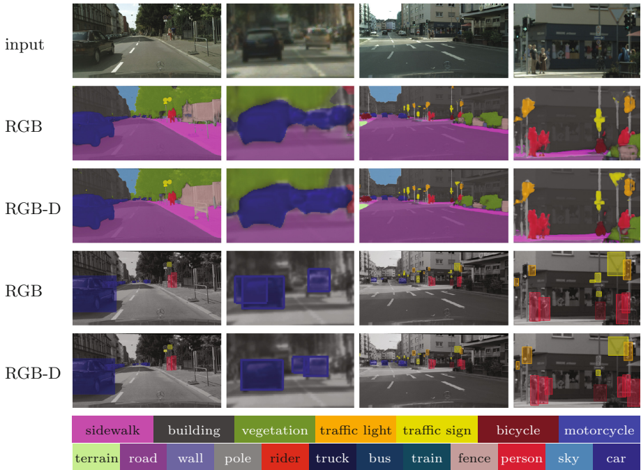
Fig. 5. Incorporating depth information (RGB-D, third line for semantic segmentation and fifth line for detection) leads to better segmentation of small objects, more details in the classification results, and tighter bounding boxes.
