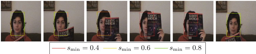
Fig. 6. The results for 3 different parameters of s_{\min} are displayed for the FaceOcc1 sequence from OTB-2015. The value of s_{\min} is an indicator of how much the object is allowed to be occluded. Lower values improve the robustness to occlusion but also require more time, since more score values need to be computed. For s_{\min} = 0.8 , the object is not detected for the third to fifth image, while for s_{\min} = 0.6 it is lost for the fourth and fifth image. However, all approaches recover when the occlusion ends.
