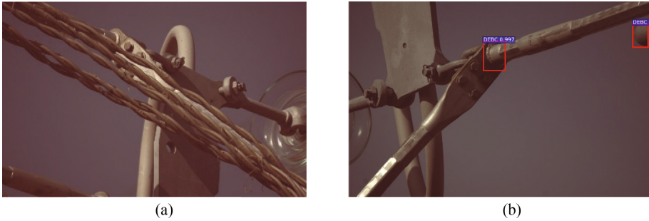
Fig. 7. Failures in detection. (a) Occluded DEBC not detected. (b) False positive DEBC detection
