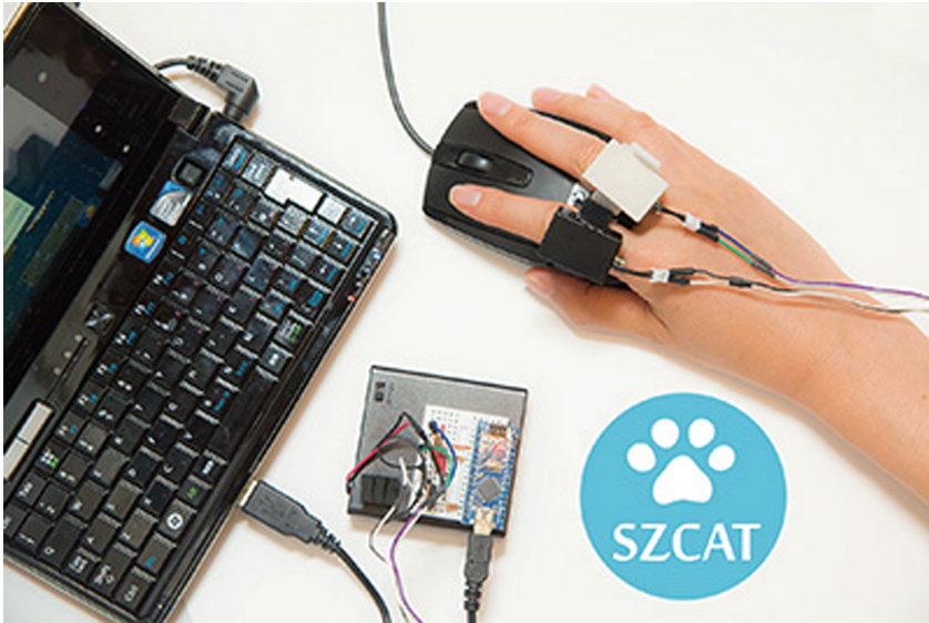
Fig. 2. An overview of vibration ring devices and its controller.
