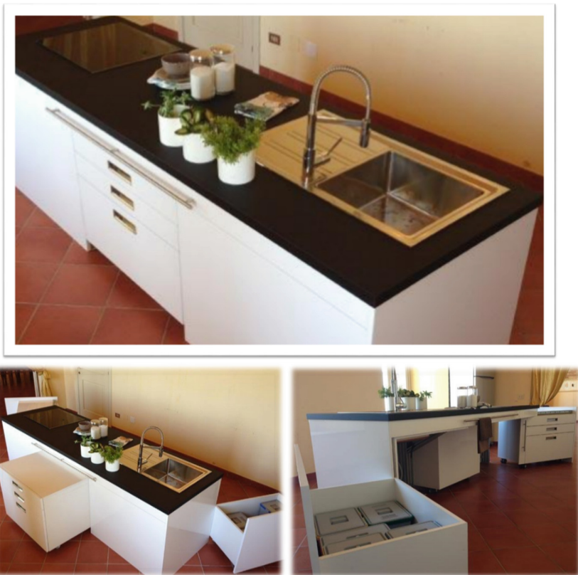
Fig. 9. Example of solution that allows people in wheelchair to access the countertop
