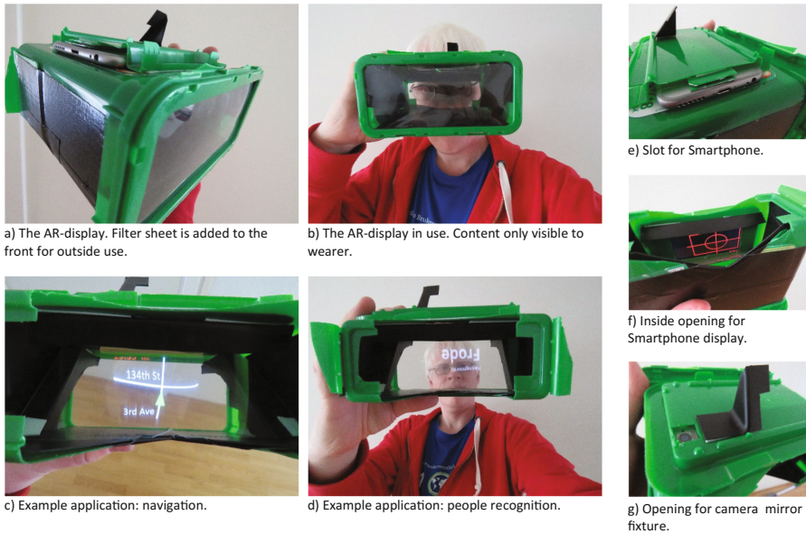
Fig. 4. The homemade wearable augmented reality Display. (a) the overall device, (b) the augmented information is not visible to onlookers, (c) and (d) augmented information as seen by the user, (d) and (e) the augmented image from the smartphone and (f) camera-mirror fixture. (Color figure online)
