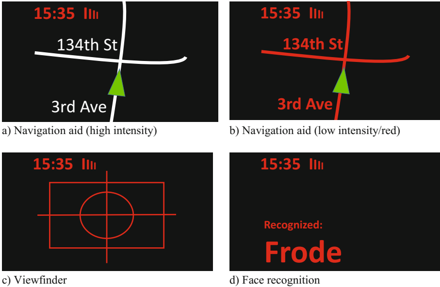
Fig. 5. Augmented information as displayed on the smartphone. Only the non-black visual elements are reflected and perceivable by the user when superimposed on the view. (Color figure online)
