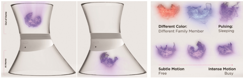
Fig. 8. Hologram projector design and essential status display patterns
